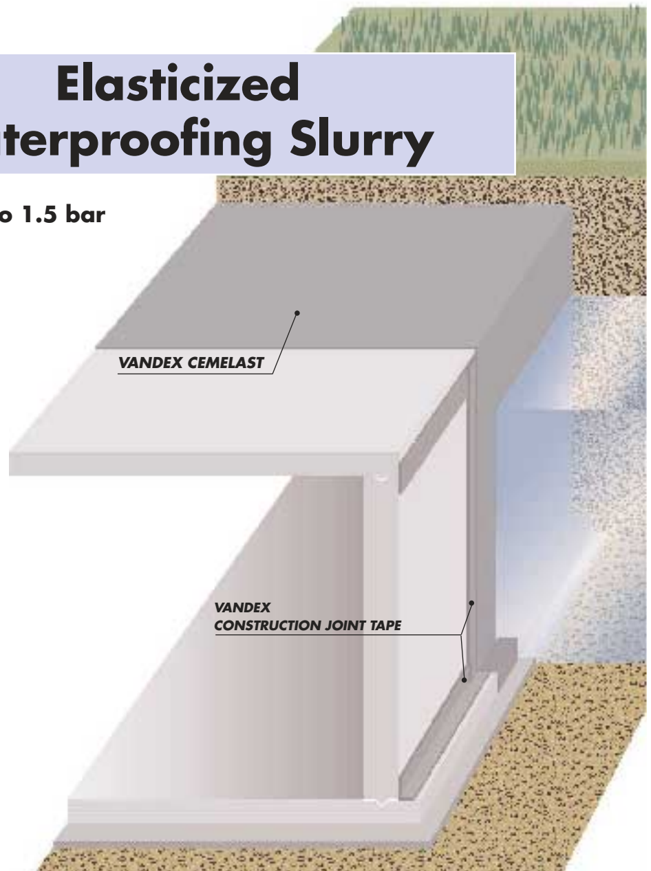
VANDEX CONSTRUCTION JOINT TAPE external application at horizontal and vertical construction joints.
